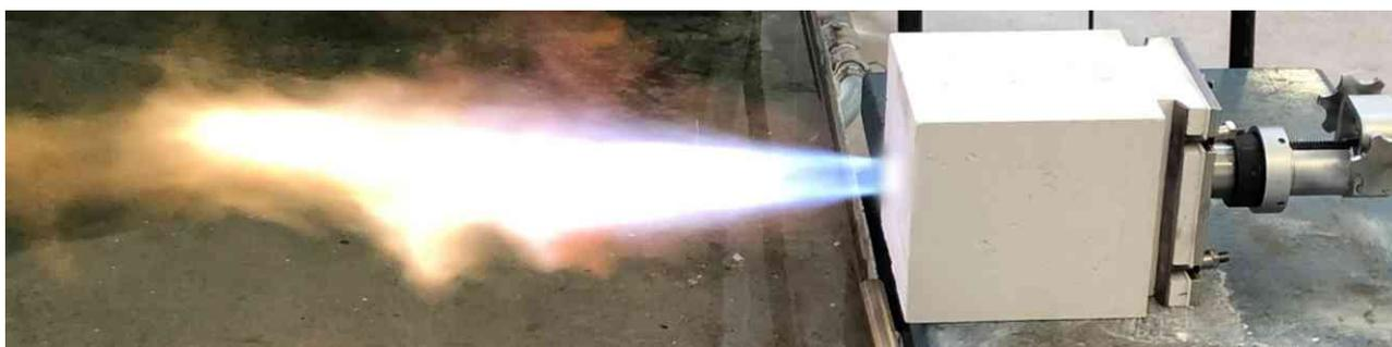
Burner operation at testing stand (flame is visible here, but a high temperature flame is nearly invisible)
