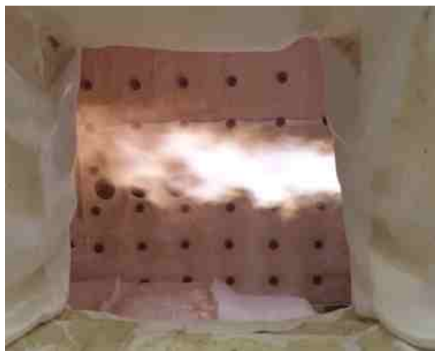
Burner operation left side is 100% natural gas/oxygen, right side is 100% hydrogen/oxygen
