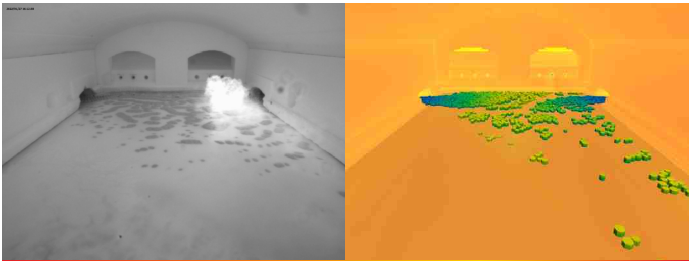
Left: image from the real furnace monitored by GS NIR camera
